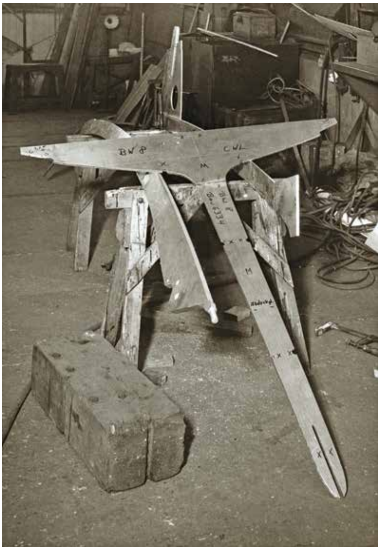
The floor at frame 8 has several important labels and cutouts to establish its location within the structure. (PEM)
