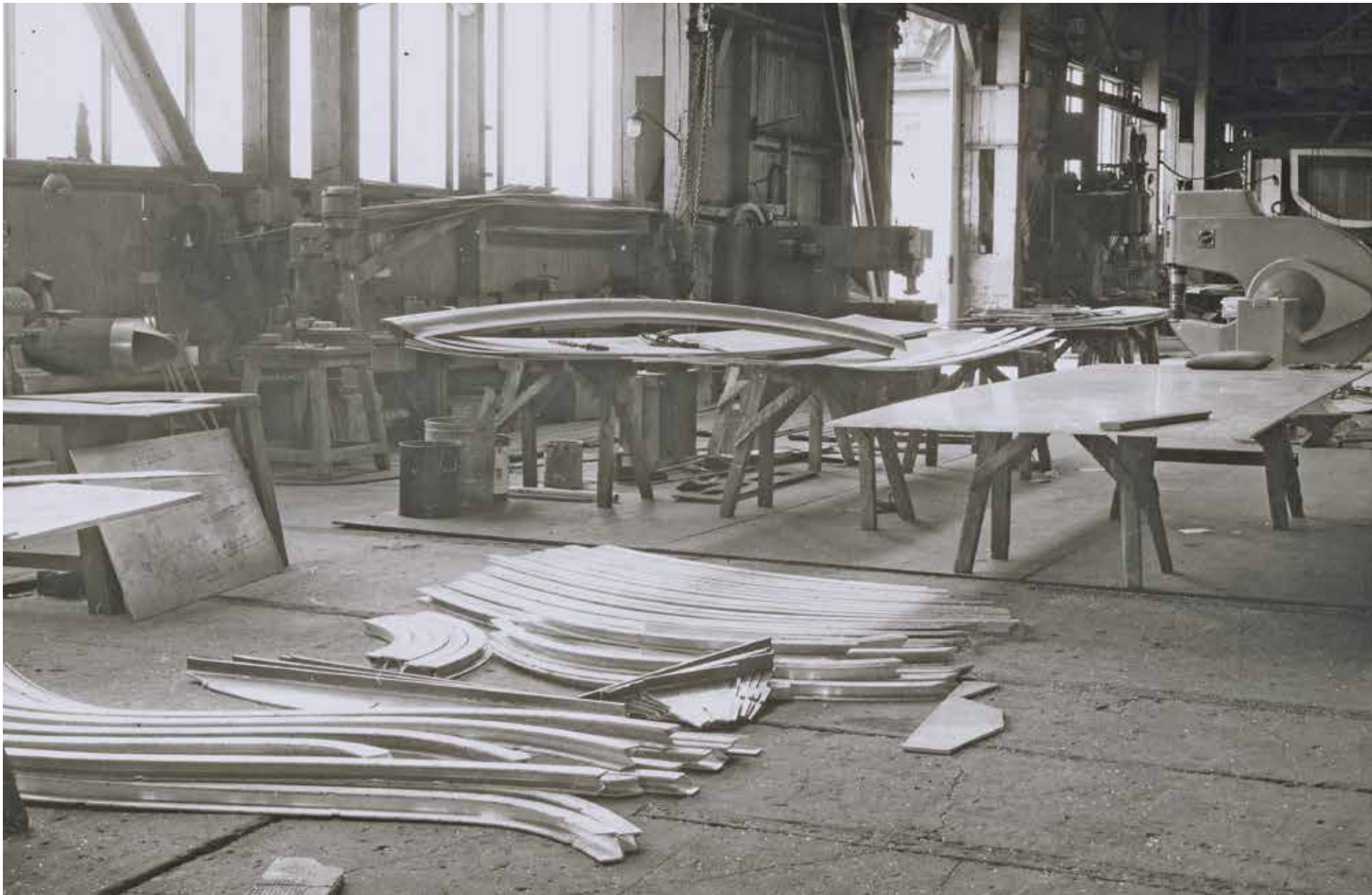
The hull frames were fabricated from flat aluminum. After they were bent into shape by the metal forming machine at right, flanges were welded to the curved webs. (PEM)
