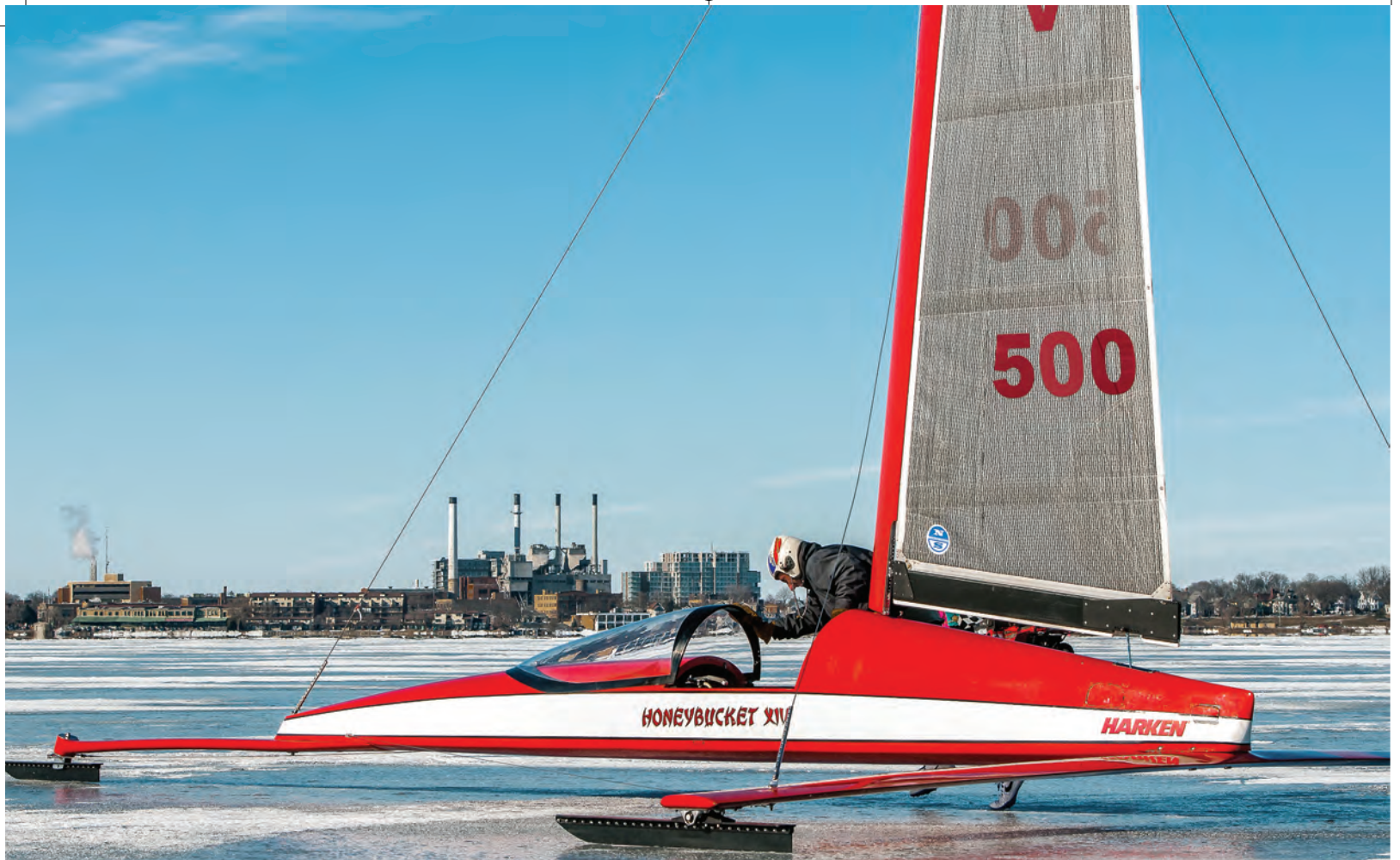
Honeybucket XIV is the last Skeeter built by Bill Mattison and is seen here being started by Harken senior engineer Steve Orlebeke. By now aero – as well as driver safety – dominated Skeeter design, along with runner development. The matching of blade and ice involves a level of voodoo comparable only with the mysteries of ‘tuning’ a go-kart chassis, tube flex providing the only suspension
