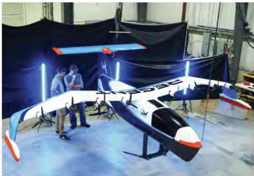
Regent’s technical demonstrator is a quarter scale seaglider prototype currently undergoing testing on the Narragansett Bay. The model’s wingspan is 18-feet (5.48 Metres) with an all-up weight of 375lbs (170kg)
