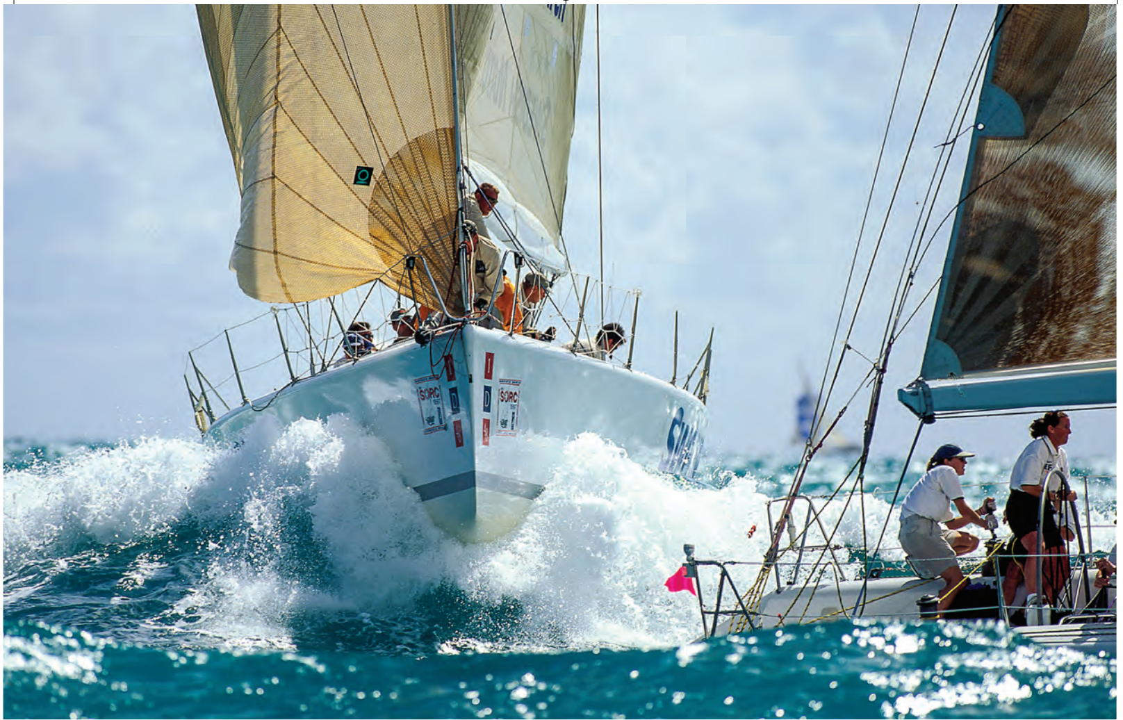
Warmer times and Van der Wal shoots the ID48 fleet in Miami in 1999. The ID48 was an early and, in retrospect, successful attempt at a big one-design capable of both regatta and distance racing – designed by Reichel-Pugh, the boats were even fitted out with a water ballast system, but this did add weight and was rarely used. They delivered very close racing, were strongly built and are still to be seen competing under IRC and ORC. Team Seahorse still has a prized trophy won in the class at this regatta – though later forced to grovel to ID48 manager John Bertrand for thoroughly destroying his mainsail in the final race on our expensive (and borrowed) yacht
